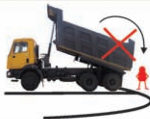
Do not stay in the working area of the tipper
